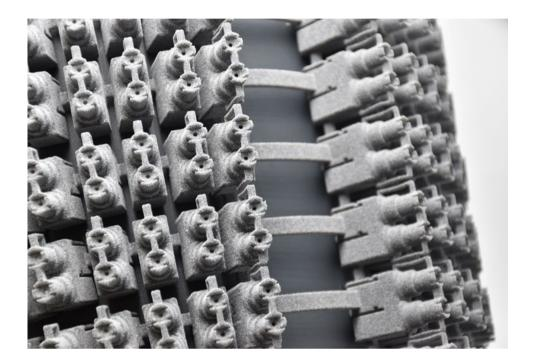
For versatility, we used MJF Ultrasint® TPU 01. Thanks to its flexibility, this material allows the belt to adapt to the user's back.
