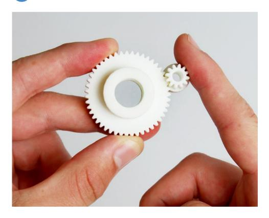
Our first models were produced using Fused Deposition Modeling.
